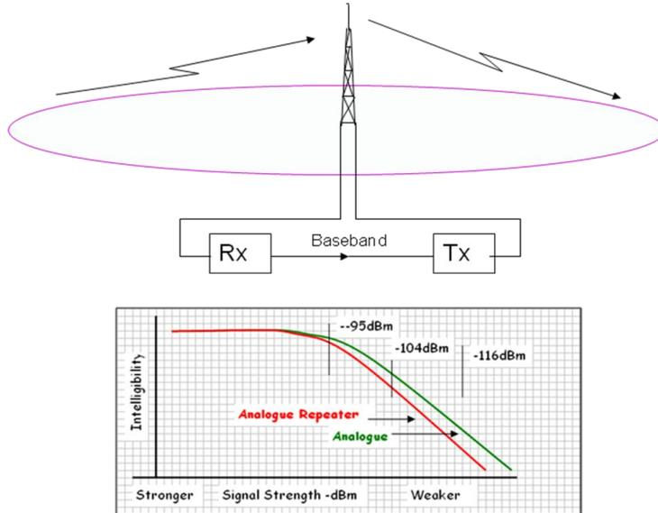
**Repeater Path from Terminal to Terminal – Analog.** Green is the path from terminal to base. Red is the combined paths, terminal to terminal
